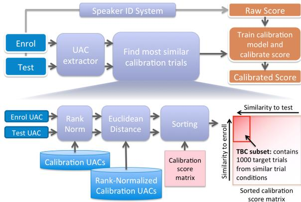
Figure 1: Flow diagram of Trial-based Calibration (TBC).
