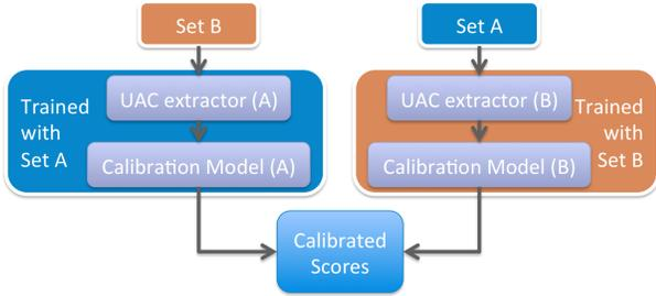
Figure 2: Cross-validation approach used in Sections 7.1 and 7.2 to highlight the benefits of Metadata calibration in the ideal scenario of matched evaluation and calibration data.
