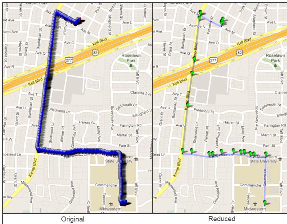
Figure 5.7. Route with set of all original points and route with the reduced interpolated set.
