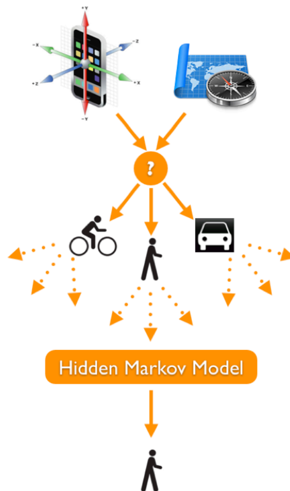
Figure 2. Overview of the algorithm utilized for the detection of the transportation mode: The accelerometer variance and the GPS speed data from the n900 are the decision tree's inputs. The decision tree classifies the input to an activity: biking, walking or driving. A hidden Markov model is fed a series of activities encountered by the decision tree. Based on the presented pattern, the hidden Markov model determines the final activity classification.
