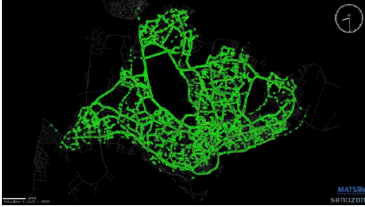
Fig. 6. Visualization of a snapshot of the simulation on MATSim's proprietary viewer; green represents the EV movements on Singapore roads
