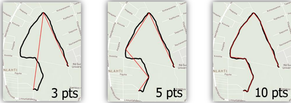
Figure 8. Polygonal approximation at three different levels. The 10-point approximation is suitable for the current zoom level. Original route has 110 points.
