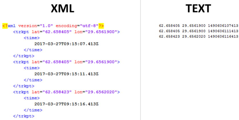
Figure 4. A route consisting of 3 points represented in XML format (left panel) and text format (right panel). The XML file contains 335 characters whereas the text file has only 104.
