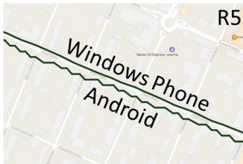
Figure 12. Two walking routes recorded on different sides of a street. The top route was recorded using Windows Phone. The lower route was recorded using an Android device, which uses lower precision to represent coordinates.
