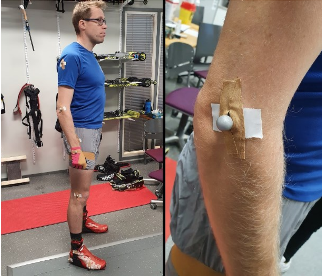
Figure 12: There were a total of 8 markers attached to the right side of the subject: in the wrist, elbow, shoulder, hip, knee, ankle, heel and base of the fifth toe. The markers are attached using sports tape.
