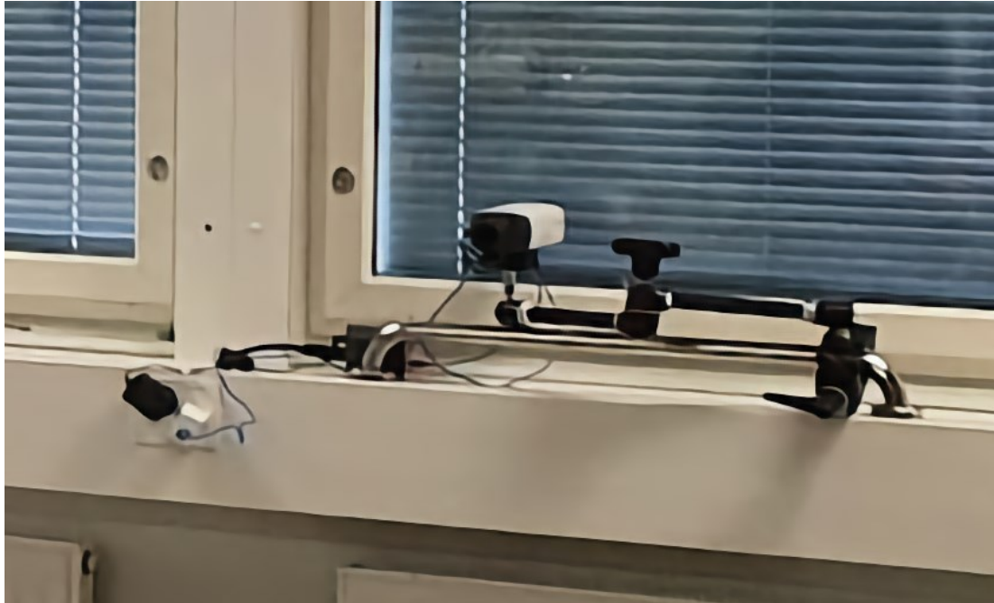
Figure 11: Lilin UFG1122ex3 camera attached to its movable arm. The easily movable arm can cause problems with calibrating VICON and the camera, since the location of the camera needs to be fixed when calibrating point cloud data to video.
