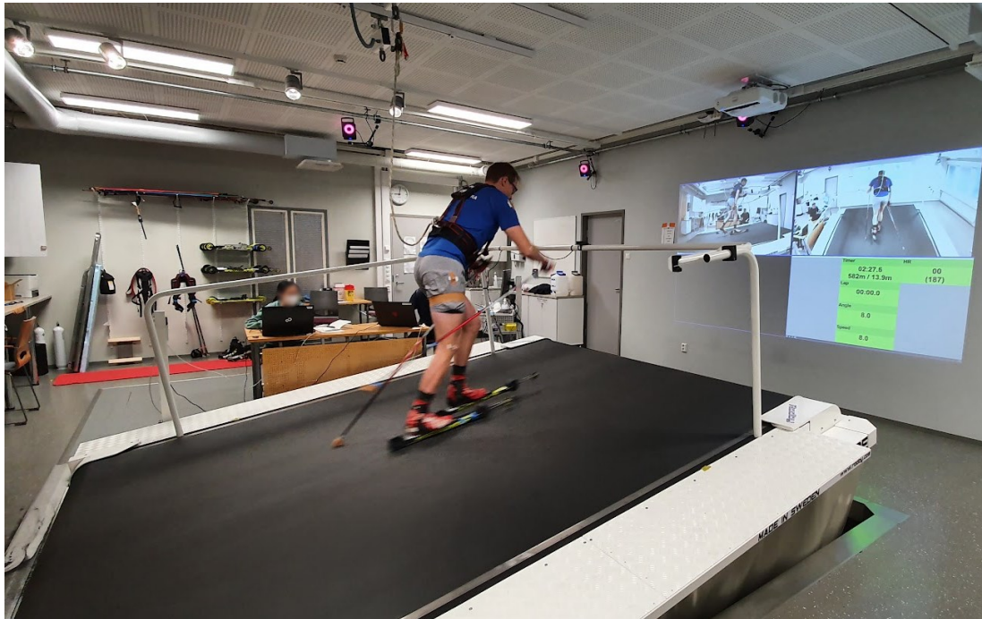
Figure 1: Athlete skiing on Vuokatti skiing laboratory treadmill during data collection event. Treadmill is set to 8° inclination.
