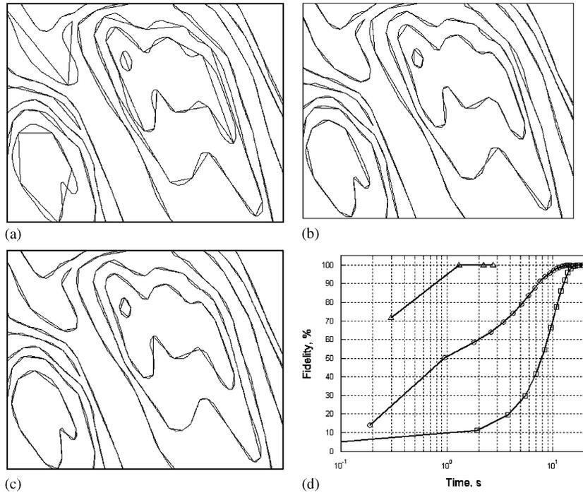
Fig. 8. Approximation results (fragment) for test data #3: (a) initial approximation with *Split-based* algorithm ( $E = 892, 158$ ); (b) initial approximation with *Merge- $L_2$*  algorithm ( $E = 173, 362$ ); (c) final result ( $E = 124, 093$ ); (d) fidelity of the approximation as a function of time. The initial solution is obtained with *Merge- $L_2$*  (triangles), *Split-based* (circles), and *Random* (squares) algorithm.
