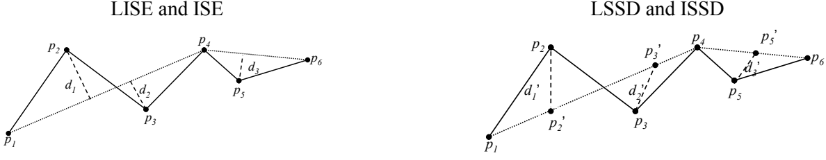
Fig. 3.1. An example of calculating ISE, LISE, LSSD and ISSD. Given P = (p_1, p_2, p_3, p_4, p_5, p_6) , and the approximated curve P' = (p_1, p_4, p_6) , where p_2', p_3' and p_5' are the approximated temporally synchronized position. ISE is estimated as d_1^2 + d_2^2 + d_3^2 and LISE is estimated as d_1^2 + d_2^2 (left). Meanwhile, ISSD is estimated as d_1'^2 + d_2'^2 + d_3'^2 and LSSD is estimated as d_1'^2 + d_2'^2 (right).
