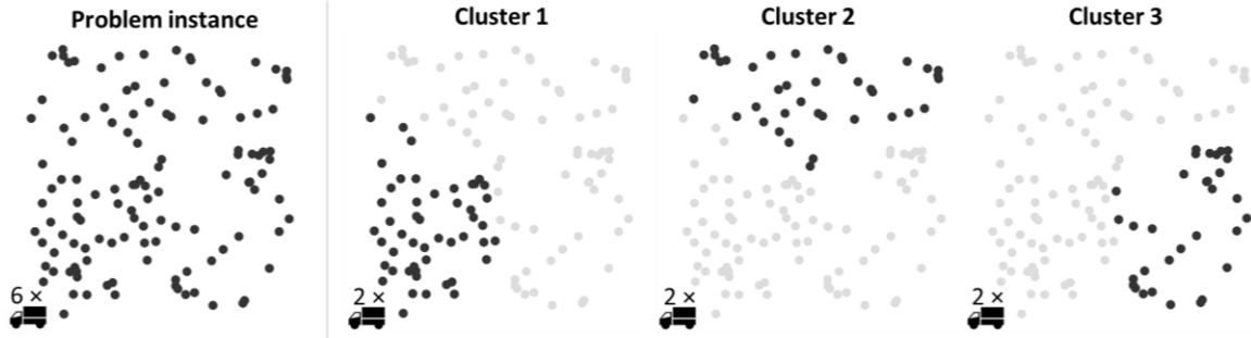
Figure 5: A VRP instance with 120 targets and 6 agents being clustered into three smaller instances where 2 agents are assigned to each. All agents start and end in the same focal point.
