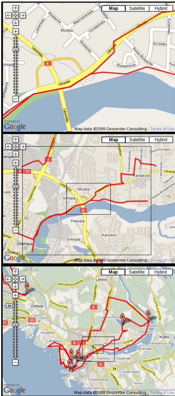
Figure 4. How the bounding box works (from top to bottom): what user sees on screen, what is drawn on map, all tracks selected.
