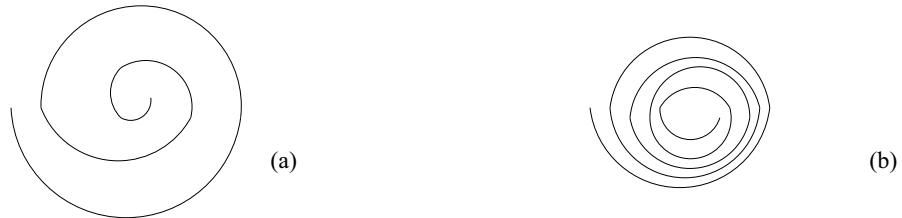
Picture 1. Lateral spring (a) no stretch (b) fully stretched
