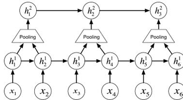
Figure 4: A pooling over time dimension of RNN
