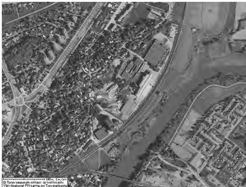
Figure 43: JPEG2000 at 0.5 bpp, MSE: 281.
