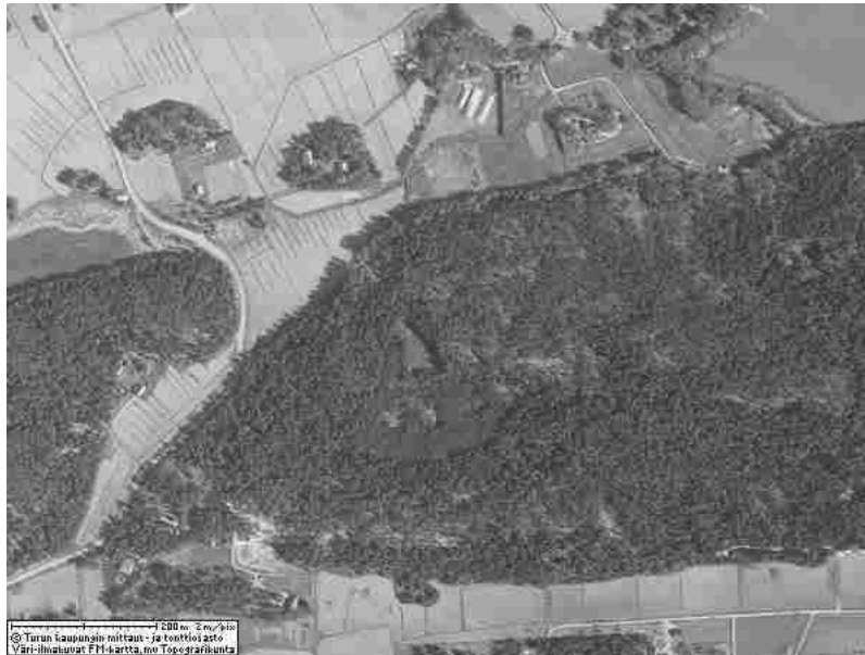
Figure 33: JPEG at 0.5 bpp, MSE: 195.
