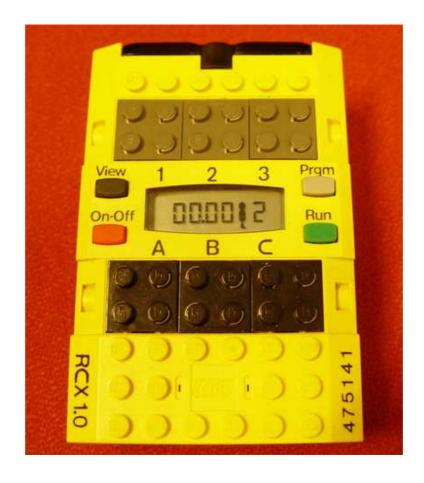
Figure 15: The RCX unit from Lego Mindstorms Robotic Invention System kit.
