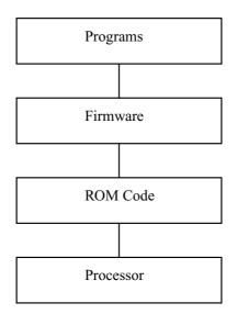
Figure 16: The logic structure of RCX unit (Laverdae, 2001)
