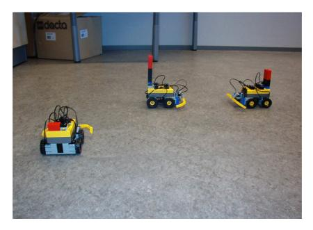
Figure 17: Robots communicating with each other during the execution of a sorting algorithm.
