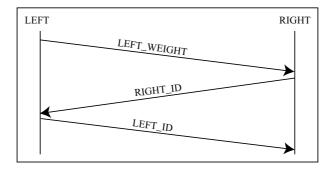
Figure 20: The part of the protocol which is used to compare the weight of the robots (González, 2004). With this protocol, robots are going to change their places.
