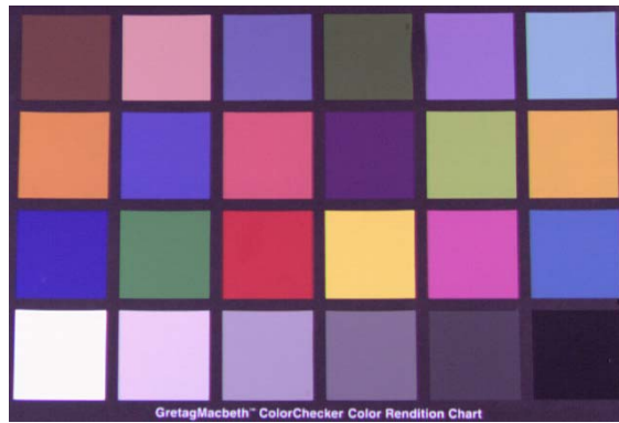
Figure 15: RGB image of Macbeth chart taken with the Minolta digital camera and 2 daylight lamps that were used also for making images of Arctic Char in 2002
