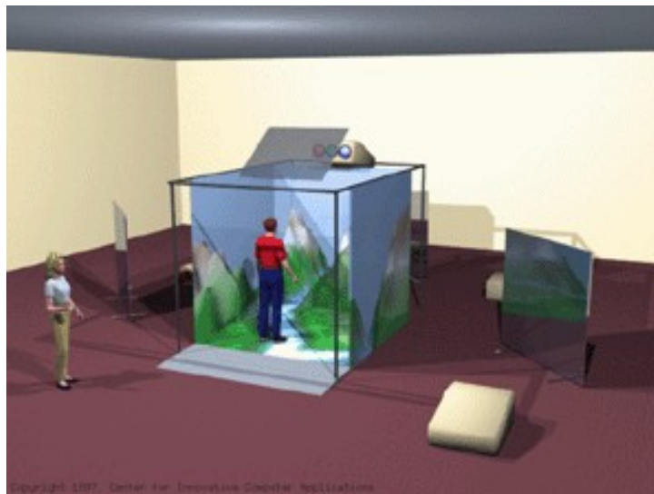
Figure 4. The CAVE system setup (ACCAD, 2005).
