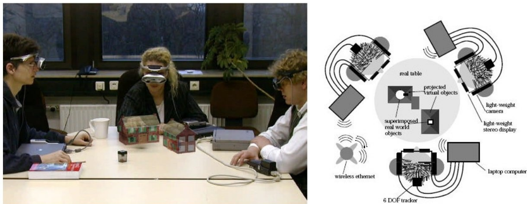
Figure 10. Virtual Round Table setup (Broll et al., 2000).
