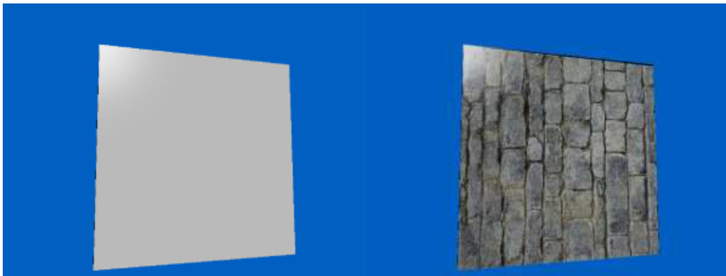
Figure 11: By textures much detail can be added to 3D models. Above is an example of how texturing brings about more realistic view of a stone wall.
