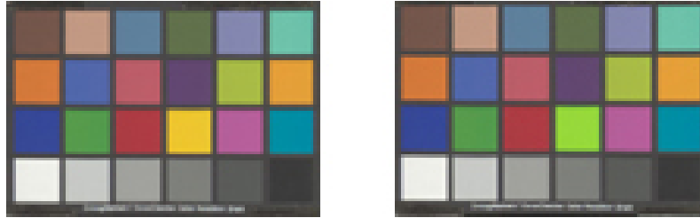
Figure 5.7: sRGB representation of the original spectral image (on the left) and the same image with a cyan filter placed over the yellow square (on the right). As a result the yellow square appears green.
