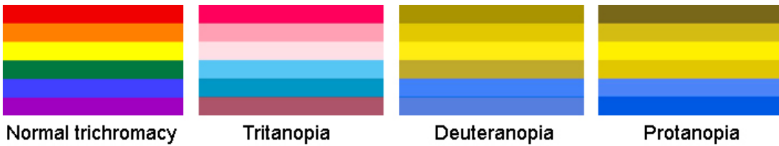
Figure 3.4: Six spectral colors, seen by individuals with different color vision (adopted from www.wikipedia.org ).
