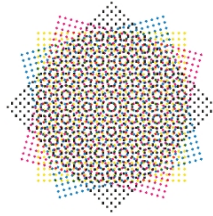
Figure 24: Traditional screen angles for color plates (Image taken from [29]).
