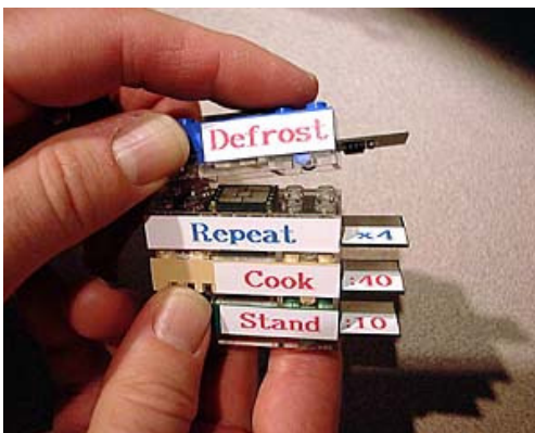
Figure 8: Tangible Programming Bricks [McN00]
