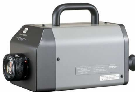
Figure 17: MINOLTA Spectroradiometer CS-1000 (Image taken from [30]).
