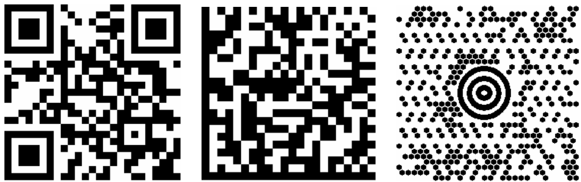
Figure 3.3. QR Code (left), Data Matrix/Semacode (center) and MaxiCode (right).
