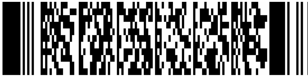
Figure 3.2. 2D barcode: PDF417
