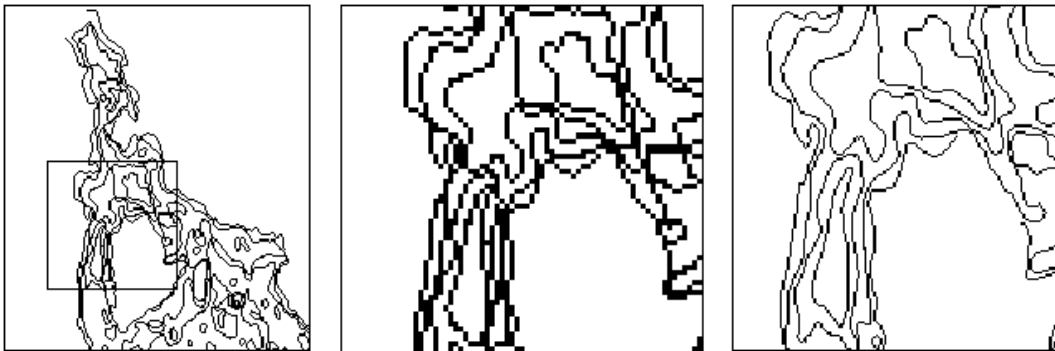
Figure 14: An example of zooming: original map (left), zooming in raster format (center), zooming in vector format (right).
