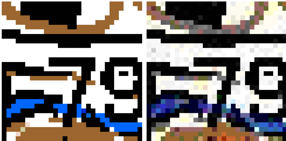
Figure 2. An example of lossy compression in a map image. On the left is the original image with 6 colors, and on the right is the JPEG-compressed image with 646 colors.
