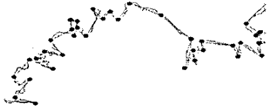
Figure 3. An example of reference lines obtained with polygonal approximation. The points of the reference line are marked with dots.
