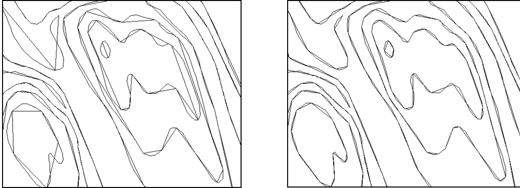
Figure 3.7.4: Approximation results for test data “Elevation map”: solution (fragment) for straightforward approach, Douglas-Peucker approximation with uniform allocation of the segments numbers (left): E_0 = 892158 , T_0 = 1.7\text{s} (left); final result (fragment) of optimal approximation with optimal number of segments after 20 iterations; E_{20} = 124093 , T_{20} = 22\text{ s} (right). The vector data reduction ratio is 5:1 ( N=38924 , M=7784 ). Processing time for full search algorithm is 157 s.
