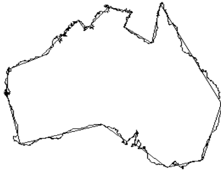
Figure 3.1.7: Min- \epsilon approximation of closed 2900-vertex contour “Australia” by M=18 linear segments.
