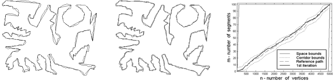
Figure 7. Result of the approximation of test data #1 with M = 100 segments using Douglas-Peucker algorithm (left), the iterative reduced search after the first iteration (middle), and the corresponding state space and the bounding corridor of width W=10 (right).
