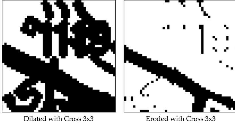
Figure 9: Dilation and erosion with Cross 3x3
