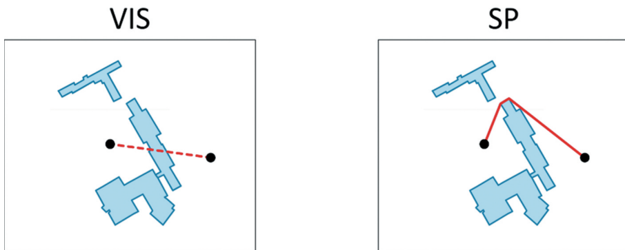
Figure 3. The way visibility (VIS) and shortest path (SP) variants handle distance calculations when buildings interfere with the line of sight.
