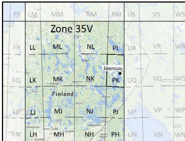
Figure 11: Map depicting a 100-kilometer grid using MGRS to locate Joensuu city in square PK of Zone 35V. [1]
