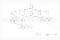
Shows the enumeration structure Edges indicate from which subset each itemset was generated
